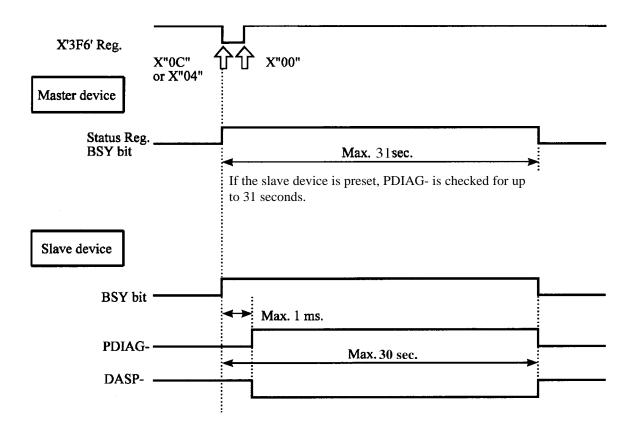
Figure 6.3 Response to software reset
